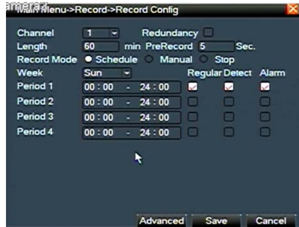
Picture 4.1 recording setup
